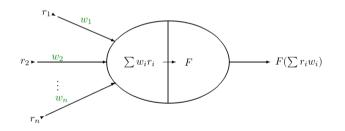
$r_i$ : real numbers, **input**  $w_i$ : real numbers, **weights**  $\sum w_i r_i$ : weighted sum F: real valued function, **activation function**
